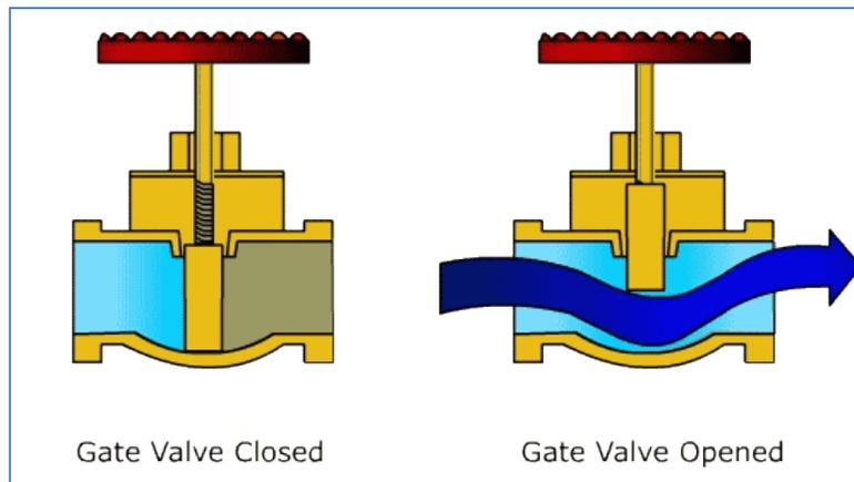
Figure 8 Gate Valves- A gate moves vertically to seal and block flow, or to open and allow liquid flow.
