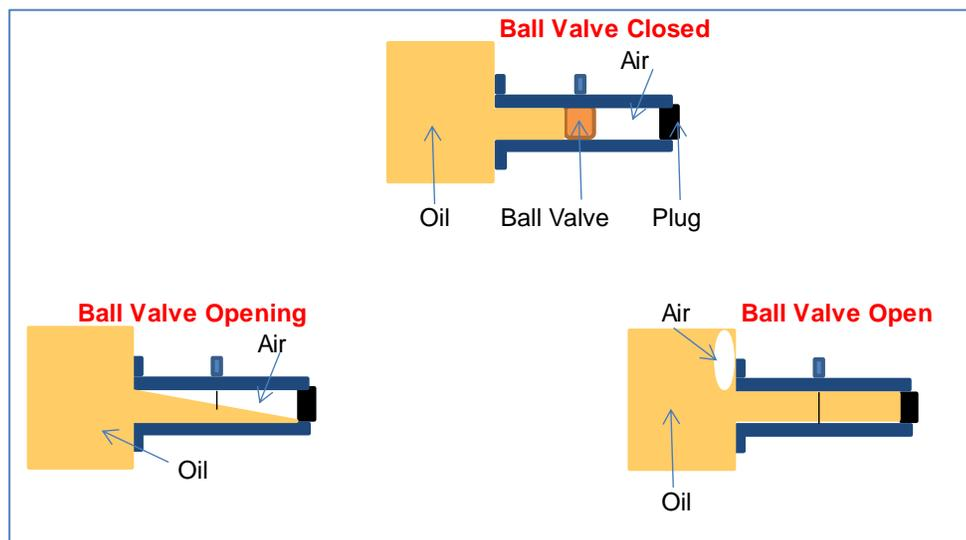
Figure 9: These sketches illustrate the danger of a gate valve when used as a transformer drain valve because when the valve outlet is blocked or connected to a closed sampling system, the trapped air moves back through the valve into the transformer.
