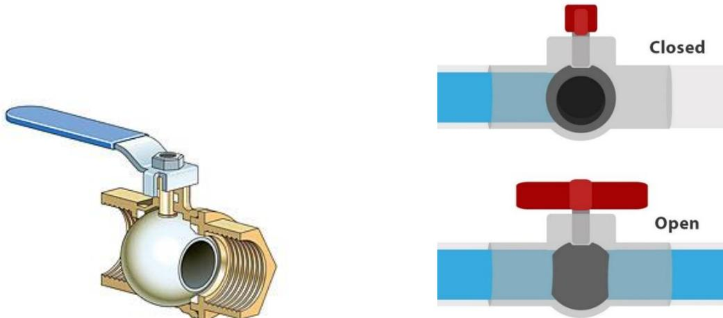
Figure 7 Ball Valves – A ball with a hole through it rotates around a vertical axis, either allowing flow, or blocking flow.
