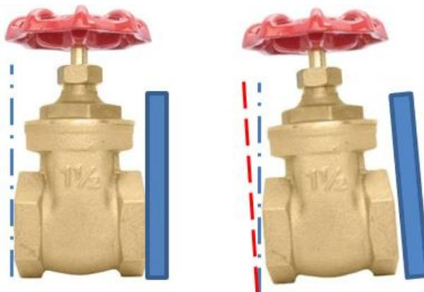
Figure 13 Blue line is vertical. Red line in second photo indicates actual angle of the valve opening face. It is not vertical, or plumb. The blue rectangle represents the tank wall on the right side of these valves.
