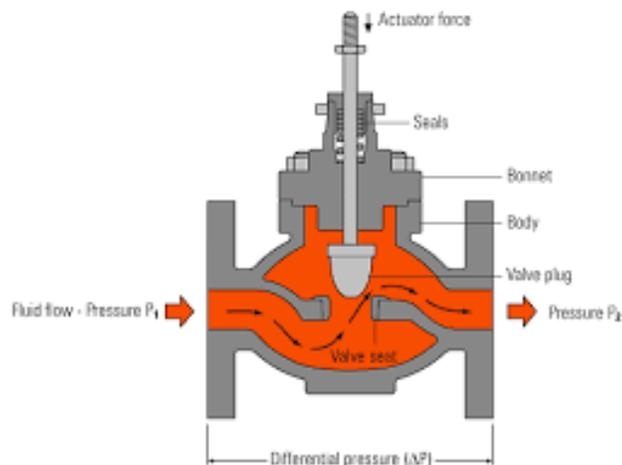
Figure 6 Globe Valve: The valve plug moves vertically to open, allowing liquid flow from input to output side, with vertical movement of the liquid through the valve seal. Source: spiraxsarco.com
