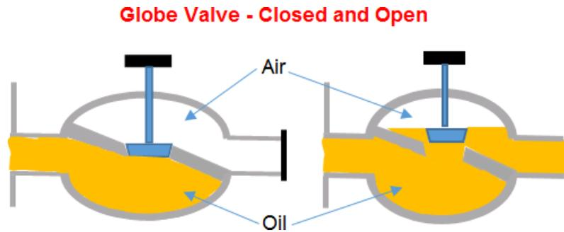
Figure 11: There is minimal danger with a globe valve used as transformer drain valve because the trapped air (white) floats above the liquid (yellow) and remains in the valve.
